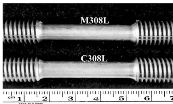
Figure 3 Modified and commercial 308L samples polished and etched with 10% oxalic acid before pre-strain tensile testing.
