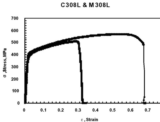
Figure 4 Stress-strain curves for modified and commercial E308L weld deposits.
