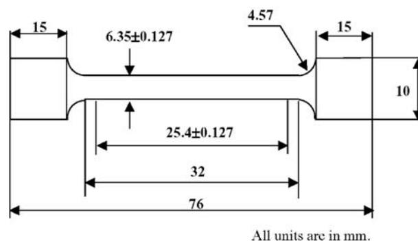
Figure 1 Schematic drawing of groove weld test pad for tension test specimen.
