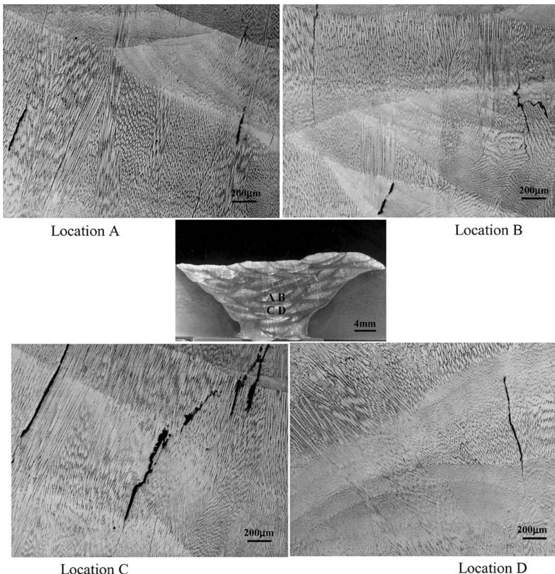
Figure 2 Microfissure morphologies on the transverse section of E308L coupon.
